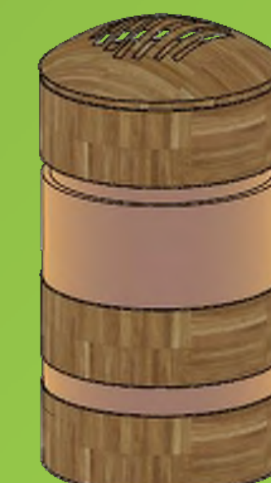
Locally Constructed Clay and Bamboo Rainwater Tank
