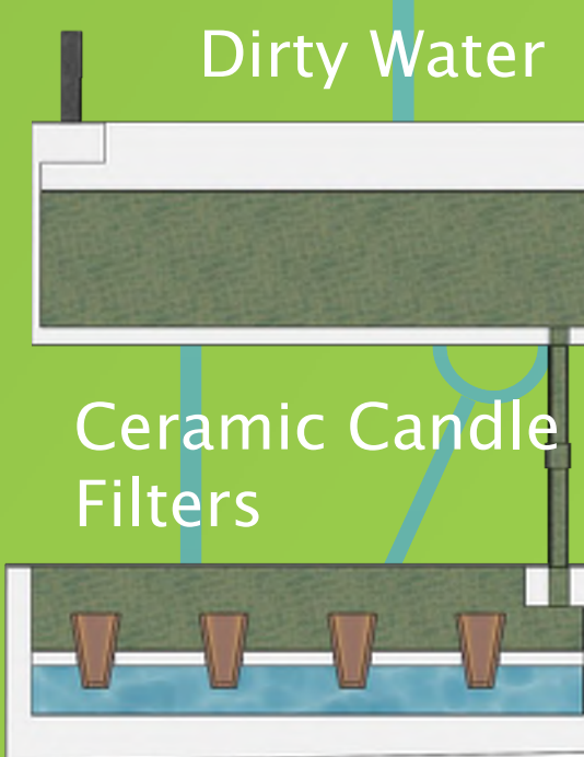
Ceramic Filters Can be Produced Locally
